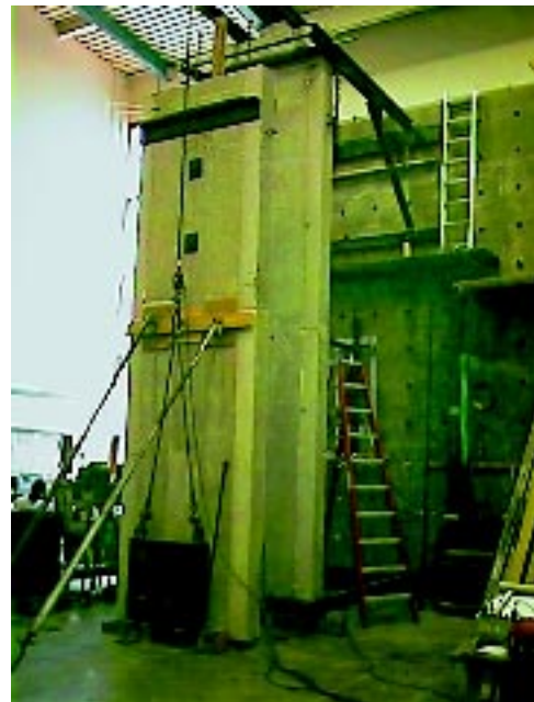
Fig. 1.12 Full-scale Slender Wall Test - combined axial and out-of-plane load.
