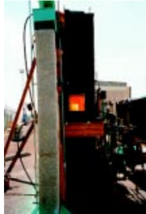
Fig.1.9 Fire rating test - ASTM E 119
