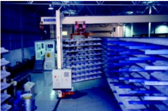
Two views of an automatic RASTRA® plant show the section where the raw elements are molded (top) and a part of the curing section with a fully automatic transport "robot" (bottom).
