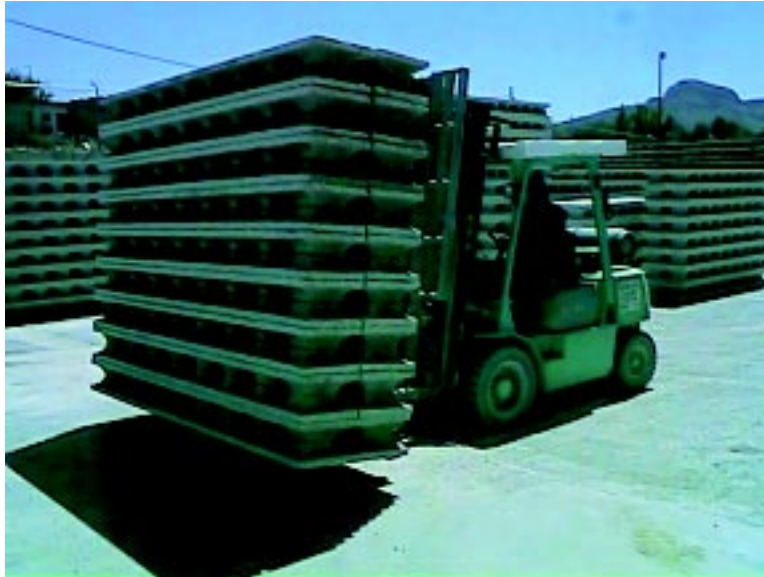
Figure B.4 RASTRA® elements moved by forklift with custom rack.
