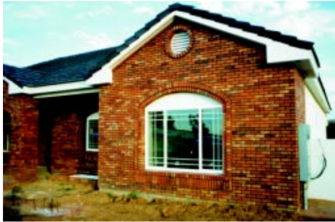
Figure 6.7 Brick veneer finish on RASTRA® home.
