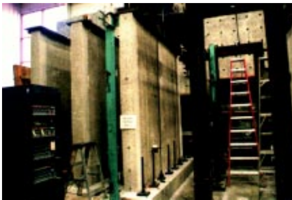
Fig. 1.11 Full-scale Shear Wall Tests - combined axial and in-plane shear loads.
