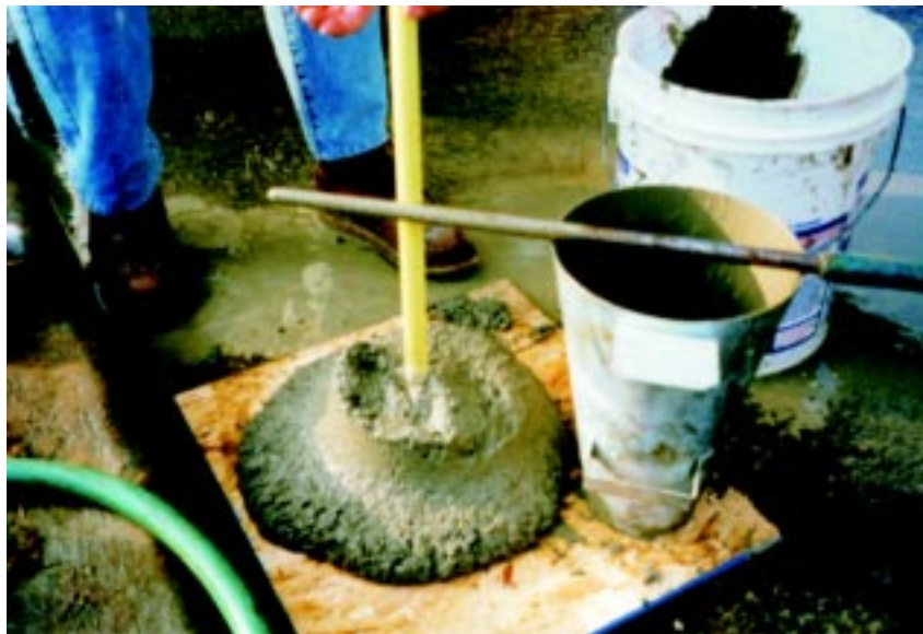
Figure 5.43 Slump range is 8 1/2" \pm 2".
