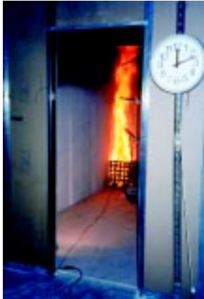
Fig.1.8 Corner burn test - elapsed time UBC 26-2
